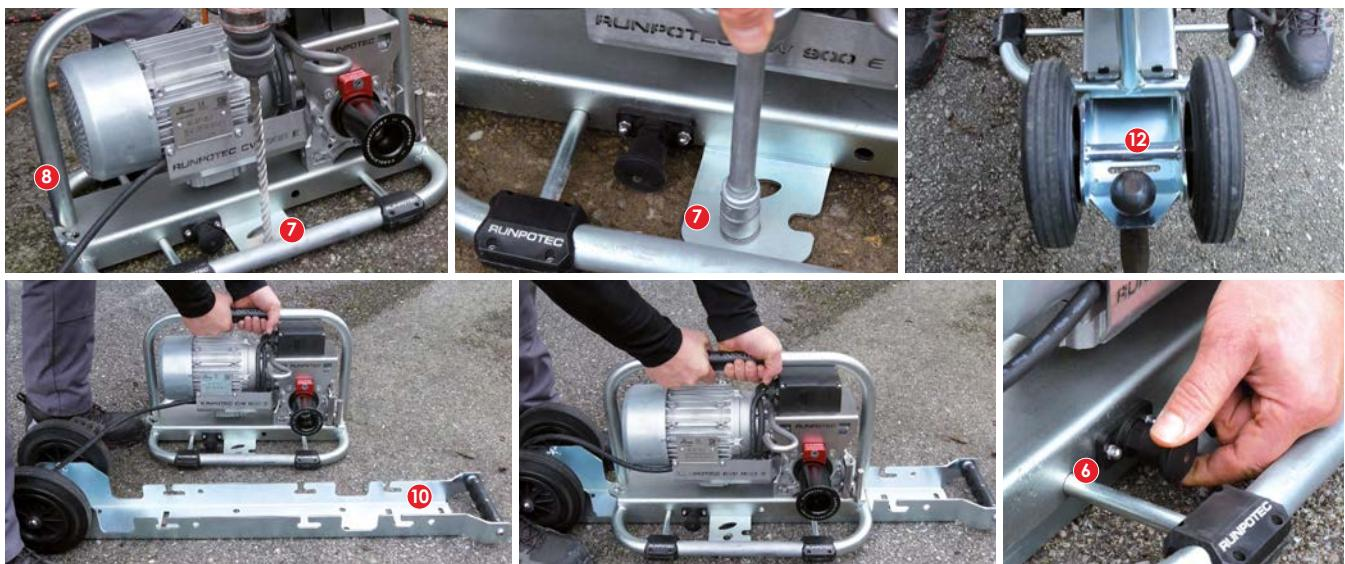
The housing can be screwed to the floor **7**, or with a strap and suitable accessories through the attachment eye **8** fixed to a solid object (e.g., tree). You can also fix the housing on the RUNPOTEC trolley **10** by means of locking bolts **6** on the rail. The trolley itself can be screwed down, hung directly on a trailer hitch **12** or fixed with a strap through the attachment eye to a fixed object.
