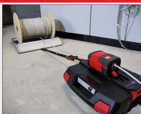
RUNPOMETER RM35 with **connecting pad and belt** fixed to cable drum roller PRO
